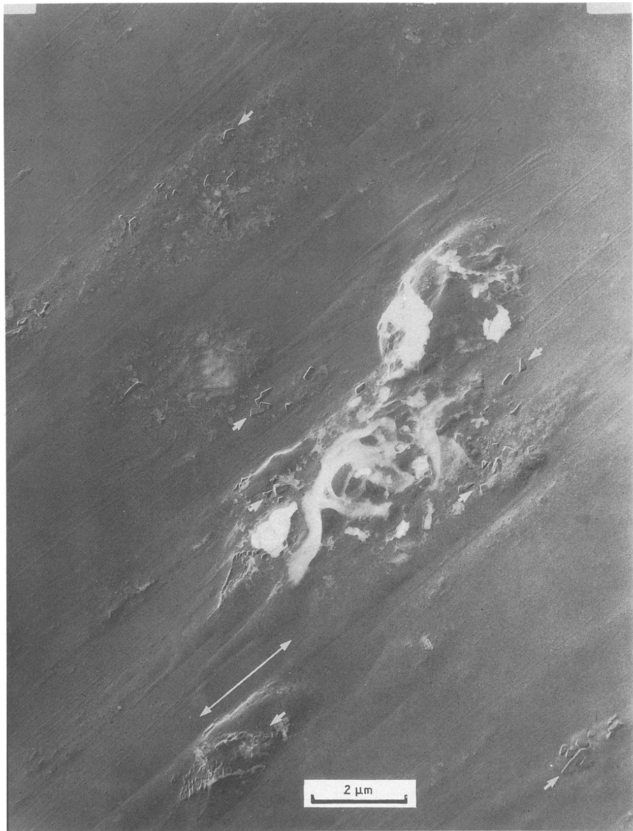
Figure 7 UHMWPE transfer film near the end of an oscillatory wear track. The tracks of transfer can be seen to end in the upper right corner. The accumulations of polyethylene on the surface contain some plate-like particles (see short arrows). The long dimension of these plate-like particles ranged from 112 to 784 nm and had an average length of 319 \pm 162 nm ( n = 20 ). This surface was replicated as in Fig. 5 and tilted 40^\circ towards the top of the figure. The light regions result from the mass-thickening effect of polymer still adhering to the replica when it was imaged.
